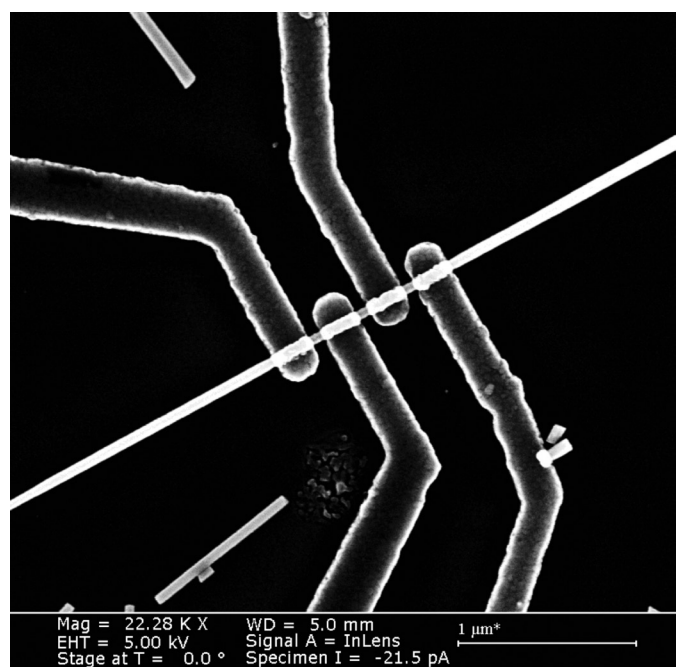
Fig. 3 SEM image of an InAs nanowire connected to four Ti/Al superconductor nanofingers. The gap between consecutive electrodes is about 50 nm.
