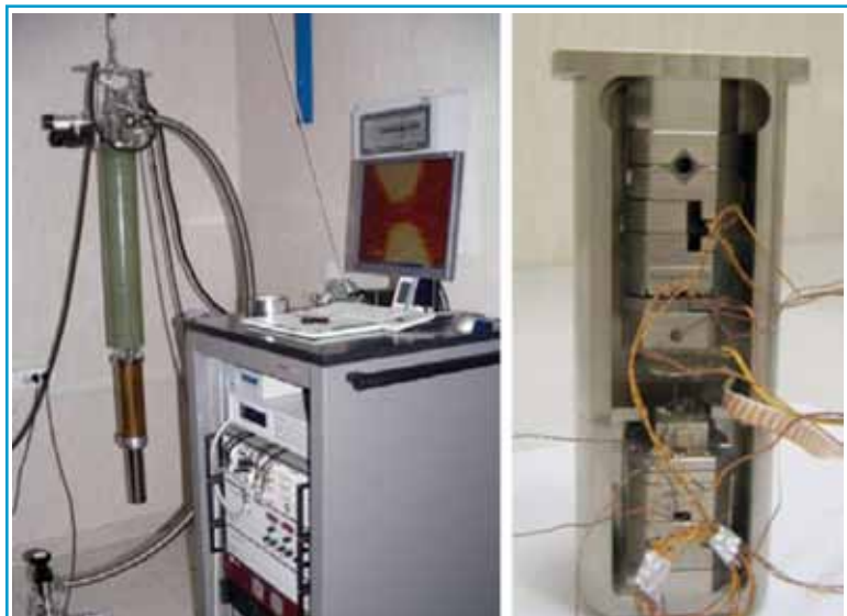
Fig. 1 (a) The new SGM lab at NEST. (b) The AFM head for SGM measurements.
