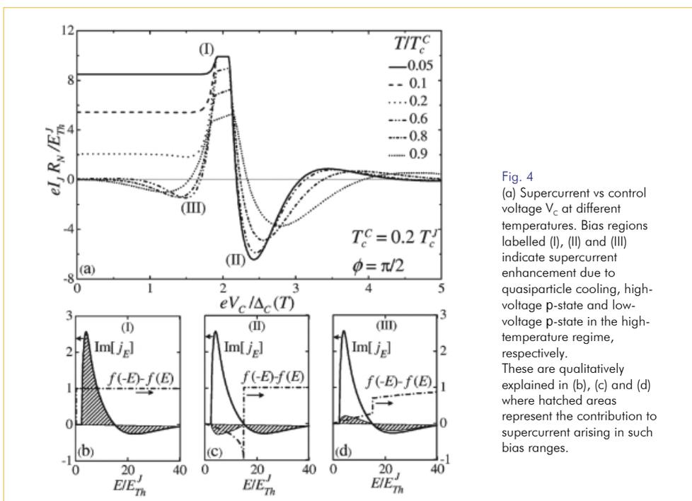
**Fig. 4** (a) Supercurrent vs control voltage  $V_C$  at different temperatures. Bias regions labelled (I), (II) and (III) indicate supercurrent enhancement due to quasiparticle cooling, high-voltage p-state and low-voltage p-state in the high-temperature regime, respectively. These are qualitatively explained in (b), (c) and (d) where hatched areas represent the contribution to supercurrent arising in such bias ranges.
