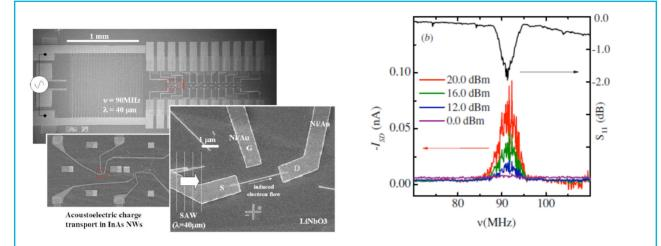
SAW-pumping in InAs nanowires. (a) SEM micrographs at incremental magnifications of one of the studied InAs NW FET structures. The 90MHz SAW is induced by means of an interdigial transducer visible on the left side of lowest magnification picture. The NW device is fabricated on the SAW propagation path. (b) Acoustoelectric current measured at room temperature; the SAW resonance is visible on the top part of the plot as a reflection dip on the transducer.
