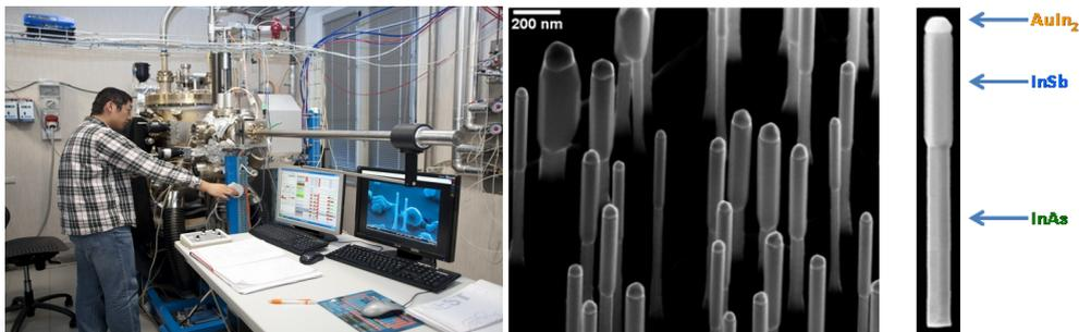
**Figure 1.** Left hand side, picture of the growth laboratory and of the Riber Compact-21 chemical beam epitaxy system. Right hand side: monocrystalline InAs/InSb NW heterojunctions recently developed at NEST. The nanoparticle catalyzing the growth process is clearly visible on the top of the NWs.
