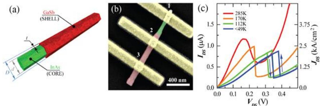
**Figure 1.** (a) Sketch of a radially heterostructured NW embedding a broken-gap GaSb/InAs junction. (b) Scanning electron micrograph of one of the studied devices, which integrate independent contacts to both the core (green) and shell (red) of the nanostructure. (c) Radial conduction displays a marked negative differential resistance, providing a clear fingerprint of bipolar transport through the broken gap heterojunction. From [5].
